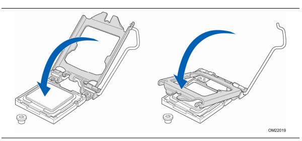
Figure 11. Lower the Load Plate
